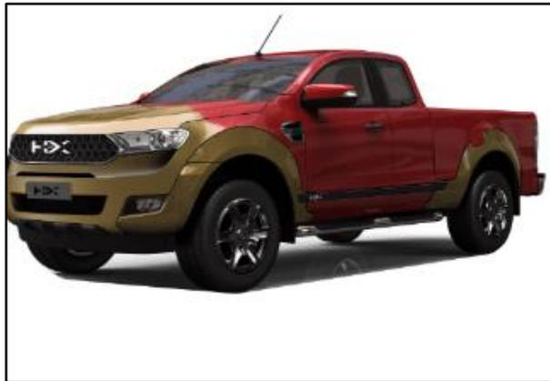
This is H2X's Warrego. The chassis is common, a Ford Ranger, with H2X replacing the power train with Fuel cells.
