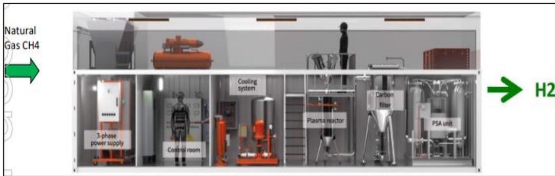
Figure 5: Conceptual methane pyrolysis production module
