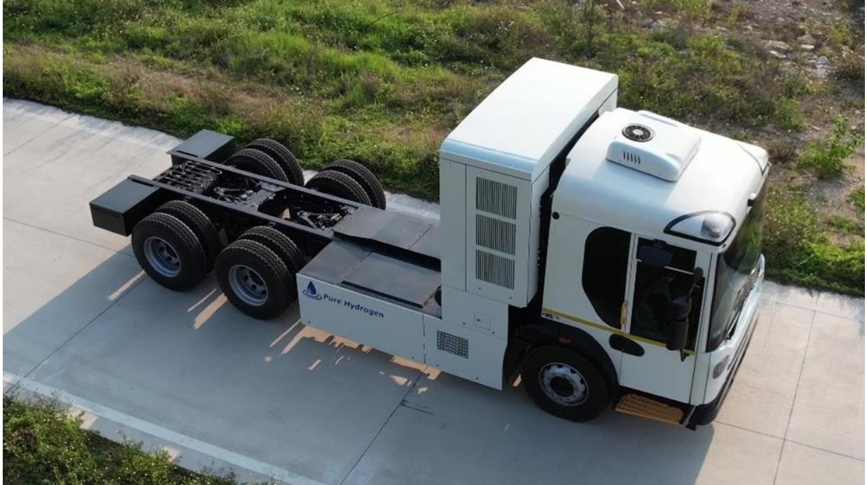
Image 4: An aerial image of Pure’s first hydrogen fuel cell waste collection vehicle, which is now being fitted with refuse collection components by Bucher Municipal.
